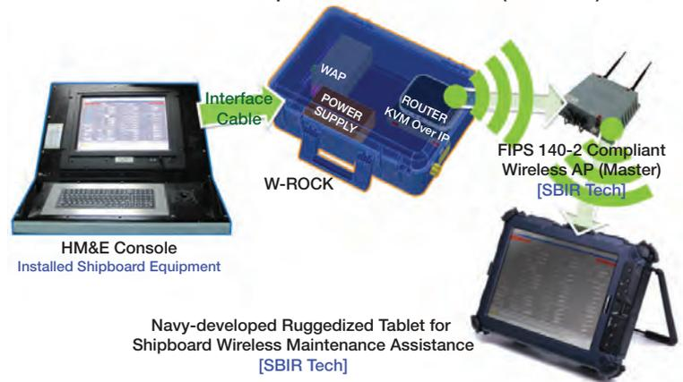
The W-ROCK system specifically supports remote operations for SmartShip console extension, data capture, documentation review/reporting, and quality management - reducing the time required to perform calibrations and maintenance by providing electronic access to:
